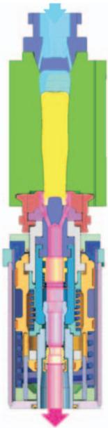
As the glass fills the finish, the vacuum also helps to cool and set the finish. With this process, the finish can be made and set with reduced settleblow. By using the vacuum to help load deeper and set the finish, the gob will flow better and easier into the finish.
