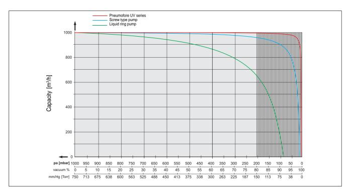
Fig. 3 - Data on capacity of vacuum pumps with changes in vacuum degree (absolute pressure)
