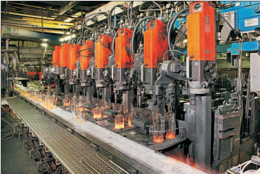
Picture 3 - IS machine in operation producing different containers (courtesy of Bottero S.p.A.)
