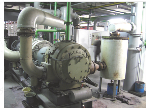
Old Wittig pump replaced by Pneumofore UV Series
