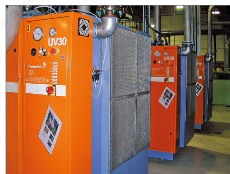
The UV30 pumps installed in 2000 worked 24/7 for 16 years
