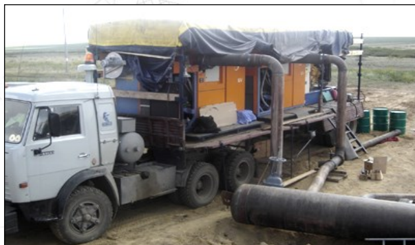
Trailer with diesel power station and UV pumps
