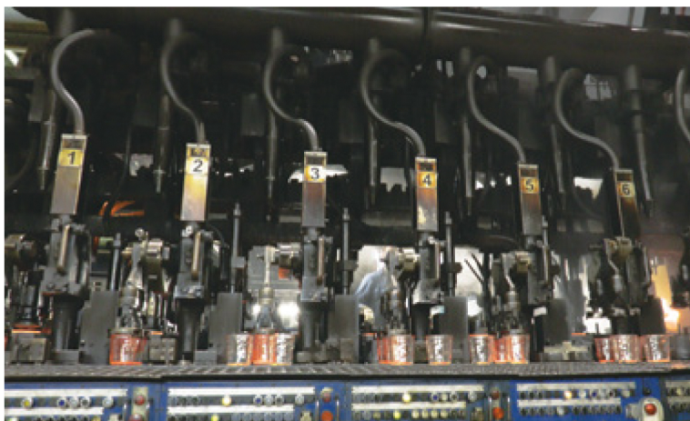
Forming of Weck glass containers at the company's IS machine.
